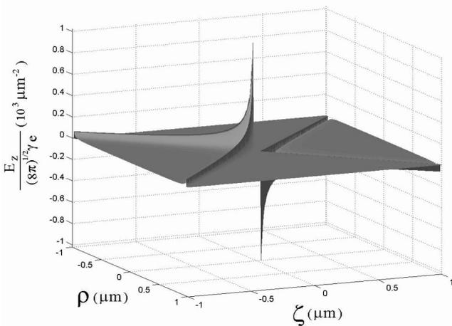
FIG. 3. Behavior of the  $z$  component of the electric field generated by a superluminal (pointlike) charge as a function of  $\rho$  and  $\zeta$ , with the same parameters as used for Fig. 1. (Once again, we skipped the points in which  $E_z$  has to diverge, namely, the vertex and the cone surface).
