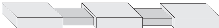
Figure 4. Two classical barriers can be constituted also by two segments of undersized waveguide, i.e., segments with a transverse size smaller than a cut-off value (depending on the frequency of the wave which travels along the waveguide). This is the set-up used in the pioneering experiment described in [8].
