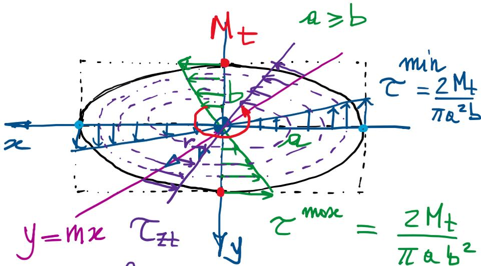
$$\frac{\tau_{zy}}{\tau_{zx}} = -\frac{b^2}{a^2} \frac{x}{y} = -\frac{b^2}{a^2} \frac{1}{m} = \cos t, \text{ lungo diametro } y = mx$$
