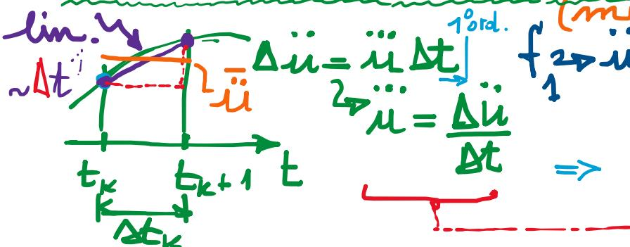
$$\begin{aligned} \Delta \ddot{u} &\rightarrow \text{media} \quad \Delta t^2 \\ \Delta \dot{u} &= \dot{u} \Delta t + \frac{1}{2} \ddot{u} \Delta t^2 \\ &= \Delta t \left( \dot{u} + \frac{1}{2} \Delta \ddot{u} \right) \end{aligned}$$
