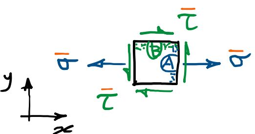
$$\left\{ \begin{array}{l} \sigma_{xx} = \bar{\sigma} \\ \sigma_{yy} = 0 \\ \tau_{xy} = \bar{\tau} \end{array} \right. \quad \begin{array}{l} \text{valori} \\ \text{assegnati} \end{array}$$
