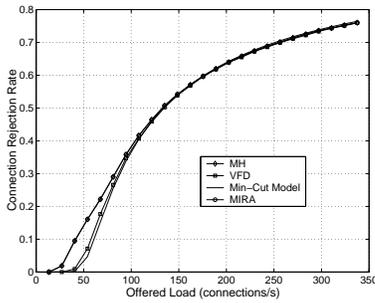
Fig. 4. Connection rejection probability versus the average total load offered to the network of Fig. 2 with link capacity equal to 60 bandwidth units and with  $N = 3$  traffic classes
