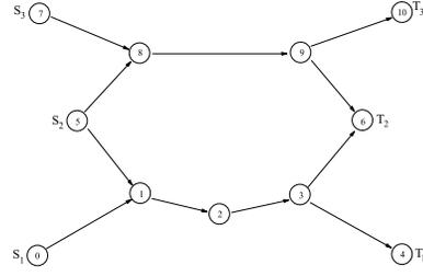
Fig. 2. Network topology with unbalanced offered load: the source/destination pairs  $S_2-T_2$  and  $S_3-T_3$  offer to the network a traffic load which is four times higher than that offered by the pair  $S_1-T_1$
