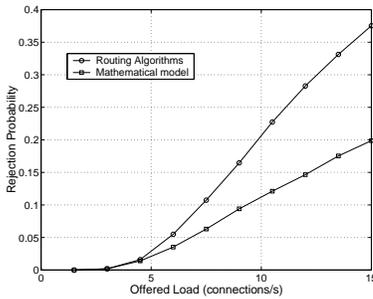
Fig. 1. Connection rejection probability versus the average total load offered to the a single link with  $b_k = 1$
