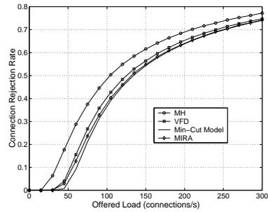
Fig. 6. Connection rejection probability versus the average total load offered to the network of Fig. 5 with  $N = 3$  traffic classes
