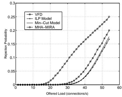
Fig. 3. Connection rejection probability versus the average total load offered to the network of Fig. 2 with link capacity equal to 24 bandwidth units
